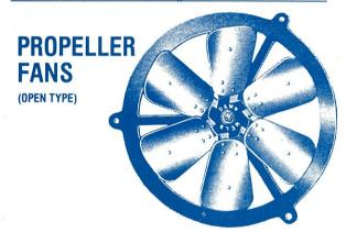
This ventilating fan is mounted on totally enclosed ball bearings, carried by three arms in a circular cast iron frame for bolting to wall or partition. The air may be impelled either inwardly or outwardly, according to the direction of rotation. Rigid streamline blades.
